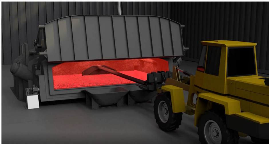
Figure 10. Skimming process with wheel loader.
